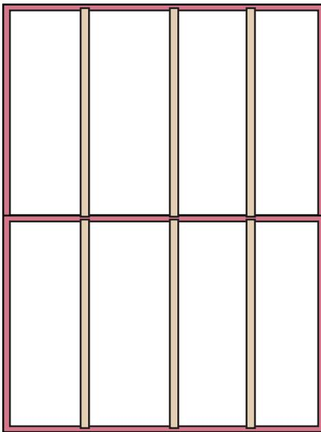
The 52 foot depth of the freight station wings was almost surely determined by the construction materials then available. Summer beams were 8” wide and 12” tall. They could not carry substantial weight for more than 25 feet. That limited their length.
